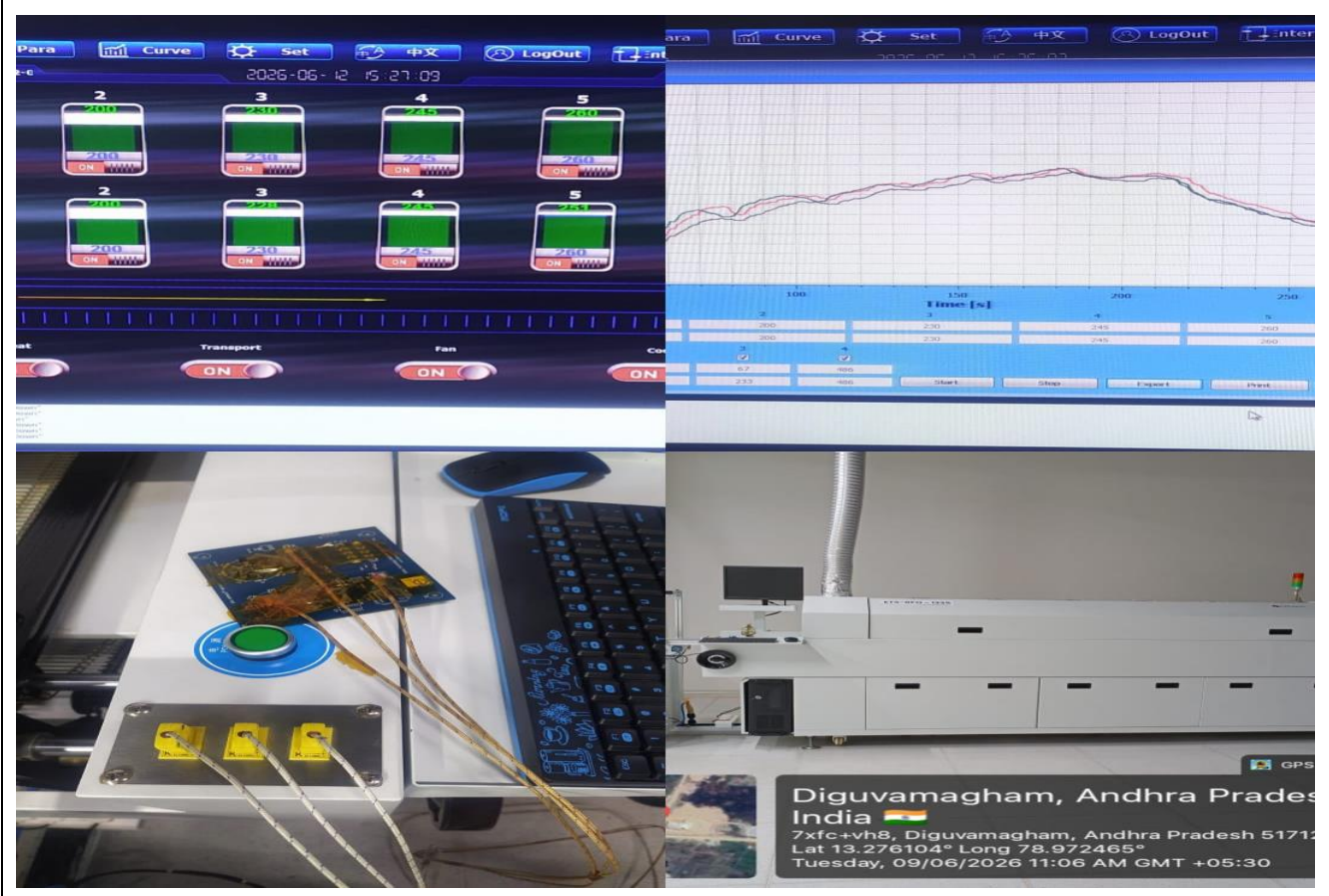
Reflow Oven: Participants studied temperature profile management and the soldering process that permanently bonds SMT components.
